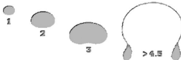
Fig.3. change in shape of raindrop with diameter
